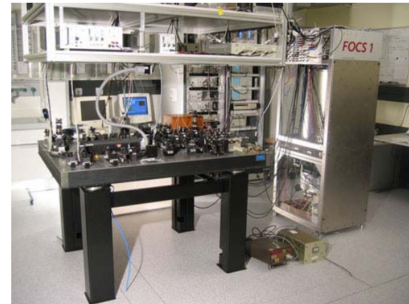
FOCS 1, a continuous cold caesium fountain atomic clock in Switzerland, started operating in 2004 at an uncertainty of one second in 30 million years (from Wikipedia)
